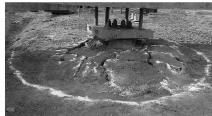
(c)基础破坏时地表裂缝
