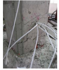
图 9 Z III -1 试件破坏形态 Fig. 9 Failure pattern of Z III -1 specimen
