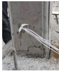
图 7 Z II -1 试件破坏形态 Fig. 7 Failure pattern of Z II -1 specimen
