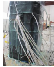
图 10 侧面纤维带鼓起 Fig. 10 Bulging of profile fiber belt
