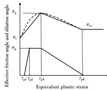
**Fig. 3 Schematic diagram of modified Mohr-Coulomb model**
