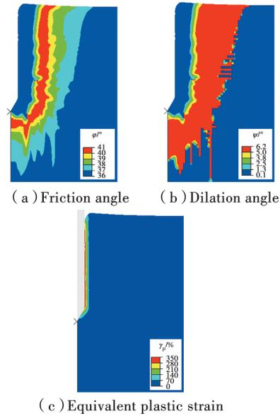
Fig. 7 Simulation results of cone penetration in KW-1 at  $z=7d$
