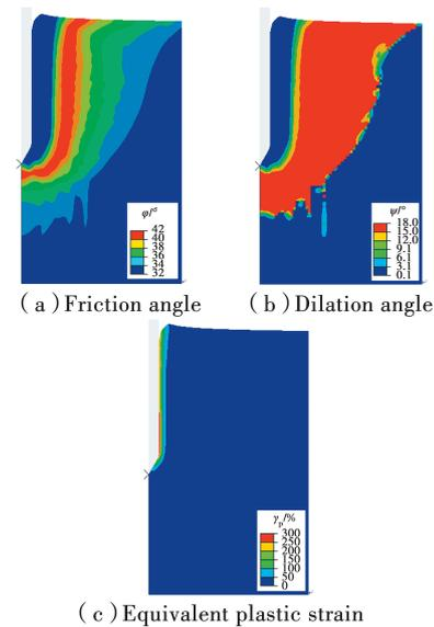
Fig. 8 Simulation results of cone penetration in UWA-1 at  $z=7d$
