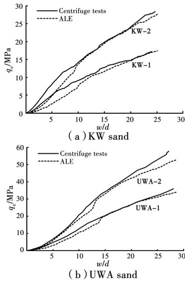
Fig. 5 Comparison between centrifuge tests and ALE results
