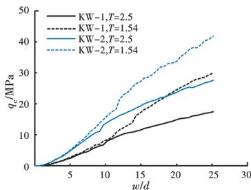
Fig. 6 Influence of stiffness degradation factor on cone resistance for KW sand
