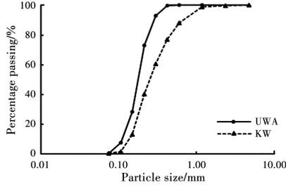
**Fig. 1 Particle size distributions of KW sand and UWA sand**
