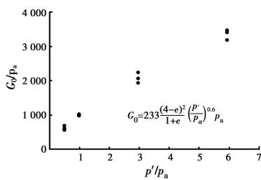
**Fig. 2 Small-strain shear modulus of KW sand**
