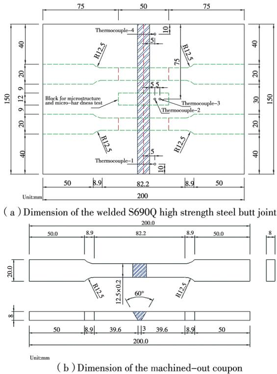
**Fig. 3 Dimension of the welded S690Q high strength steel butt joint and machined-out coupon**
