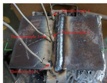
(a) Welded S690Q high strength steel butt joint
