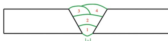
Noted: The number(1~4) represents the completion sequence of welding pass
