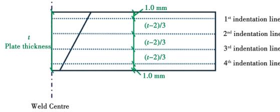
**Fig. 6 Indentation distribution on S690Q high strength steel butt joint**
