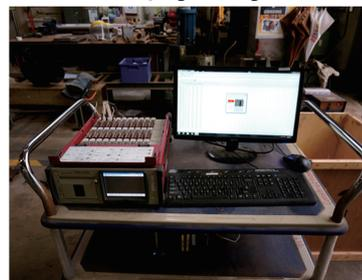
(b) Temperature measurement device
