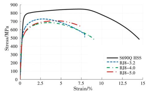
**Fig. 9 Stress-strain curves of S690Q high strength steel butt joints**
