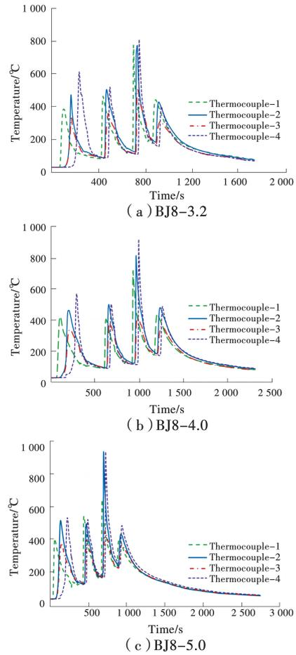
**Fig. 4 Temperature history curves of S690Q high strength steel butt joints**
