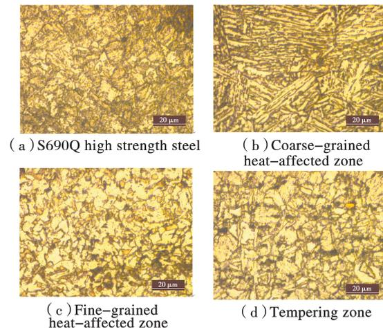
**Fig. 5 Microstructure of S690Q high strength steel, coarse-grained heat-affected zone, fine-grained heat-affected zone and tempering zone**
