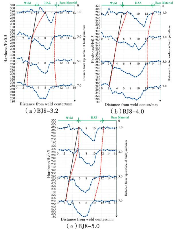
**Fig. 7 Micro-hardness distribution of S690Q high strength steel butt joints**
