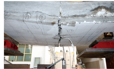
(a) 跨中断裂
