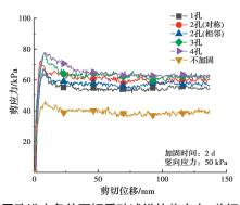
图 6 不同孔进水条件下钙质砂试样的剪应力—剪切位移曲线 Fig. 6 Shear stress-shear displacement curves of calcareous sand specimens under different water intake conditions
