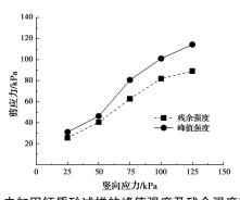
图 13 未加固钙质砂试样的峰值强度及残余强度对比图 Fig. 13 Comparison of peak strength and residual strength of unreinforced calcareous sand samples
