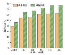
图 7 不同孔进水条件下钙质砂试样的峰值与残余强度对比 Fig. 7 Comparison of peak strength and residual strength of calcareous sand samples under different water inlet conditions
