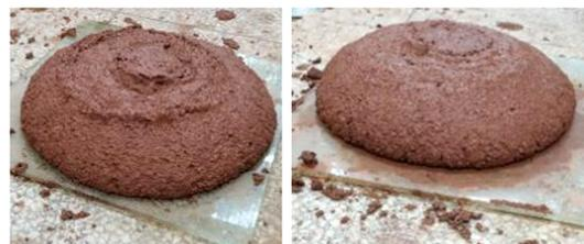
(a) 30%泥岩含量渣土 (b) 50%泥岩含量渣土
