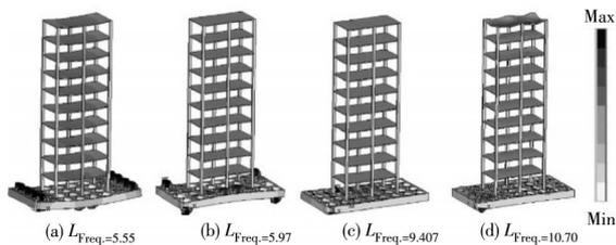
Fig. 17 Vibration modes of structures with PF at points
