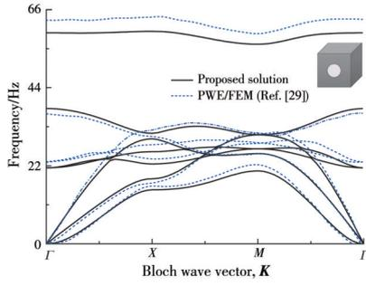
(a) The comparison between the proposed method and the method proposed by Qian et al.<sup>[29]</sup>
