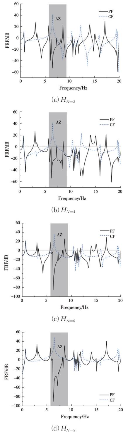
**Fig. 10** Frequency response curves of observation points  $H_{N=2}$ ,  $H_{N=4}$ ,  $H_{N=6}$  and  $H_{N=8}$  under the bending waves
