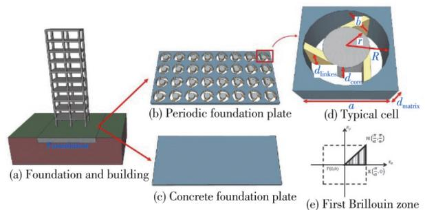
**Fig. 1 Schematic diagram of foundation with SS**
