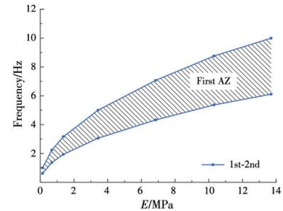
Fig. 7 Influence of the rubber elastic modulus on AZ
