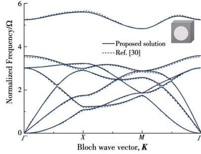
(b) The comparison between the proposed method and the method proposed by Hsu et al.<sup>[30]</sup>
