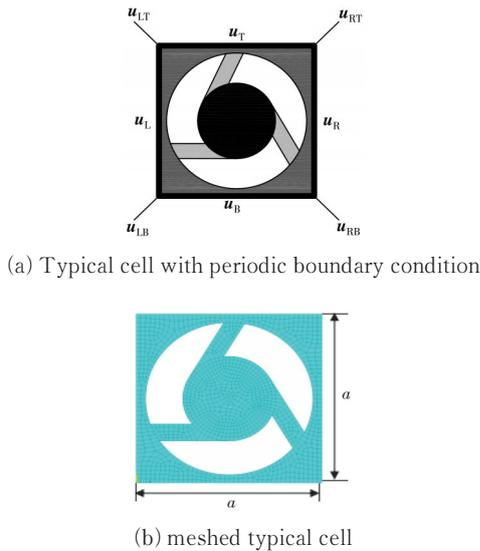
**Fig. 2 Typical cell with periodic boundary condition and meshed typical cell**
