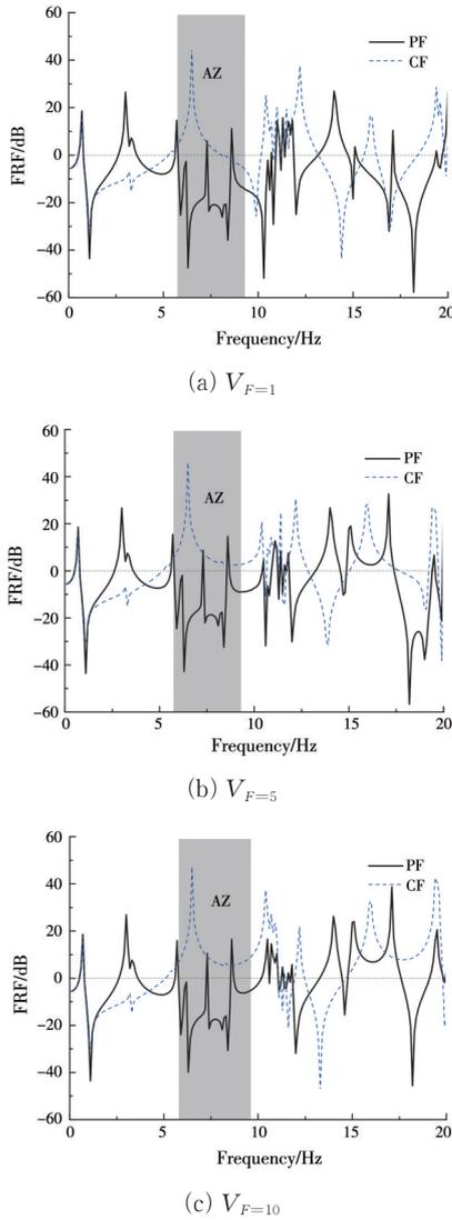
**Fig. 11 Frequency response curves of observation points  $V_{F=1}$ ,  $V_{F=5}$ , and  $V_{F=10}$  under the bending waves**
