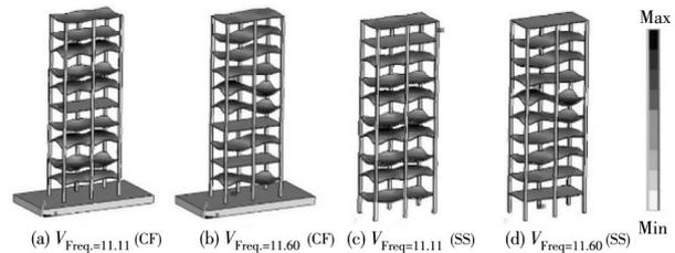
Fig. 18 Vibration modes of structures with CF at points and SS at point
