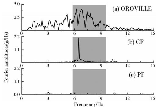
**Fig. 13 Fourier transform of acceleration response at point  $V_{F=10}$  under the Oroville wave ground motion**
