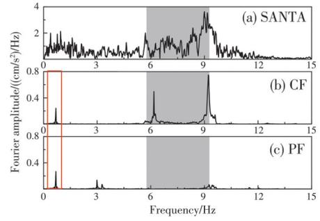
**Fig. 15 Fourier transform of acceleration response at point  $V_{F=10}$  under Santa wave ground motion**
