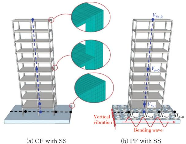
Fig. 9 CF with SS and PF with SS
