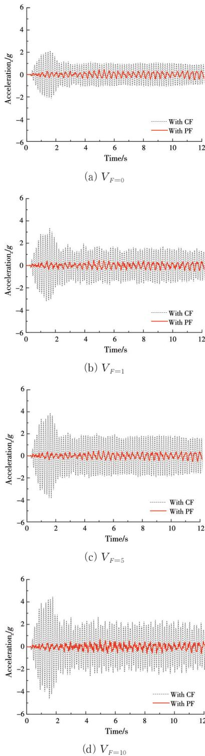
**Fig. 12 Acceleration response of vertical observation points  $V_{F=0}$  (i.e.,  $H_{N=4}$ ),  $V_{F=1}$ ,  $V_{F=5}$ , and  $V_{F=10}$  under the incident of the Oroville wave**
