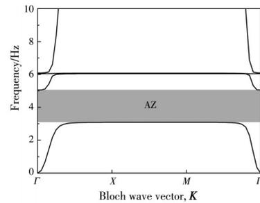
**Fig. 4 Bending-wave dispersion diagram of a typical cell**
