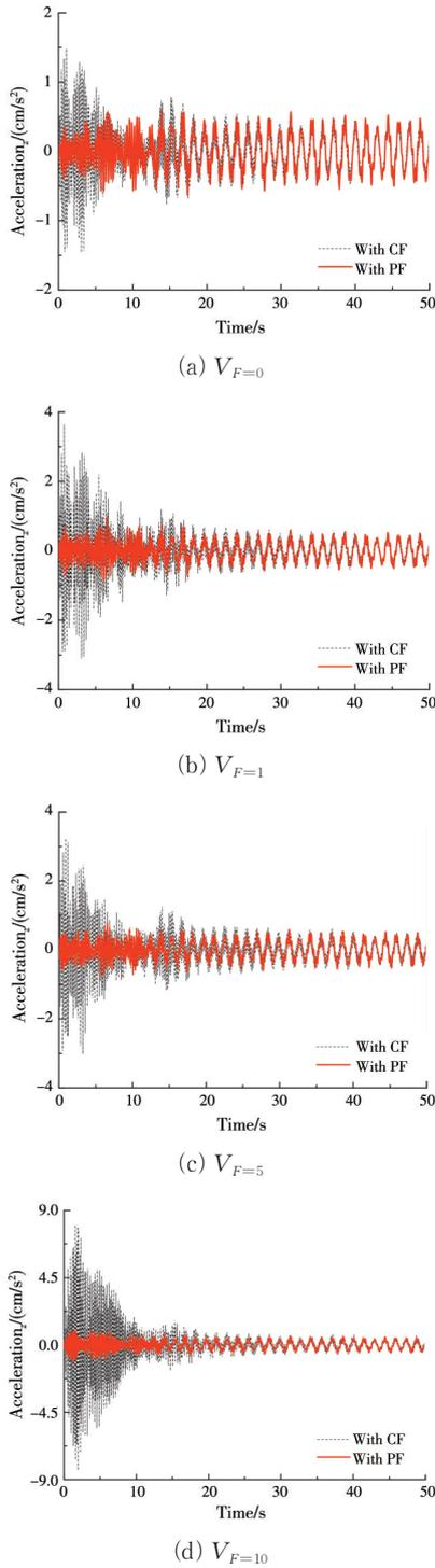
**Fig. 14 Acceleration response of vertical observation points  $V_{F=0}$  (i.e.,  $H_{N=4}$ ),  $V_{F=1}$ ,  $V_{F=5}$  and  $V_{F=10}$  under the incident Santa Felicia wave**
