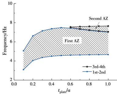
Fig. 5 Influence of plate thickness on AZs
