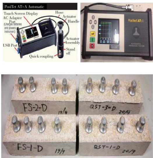
Fig. 3 Posi-Test AT-A instrument for pull-out test and dolly glued on the surface of mortar
