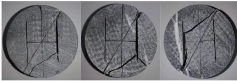
(c) 平行双裂隙试件30°加载
