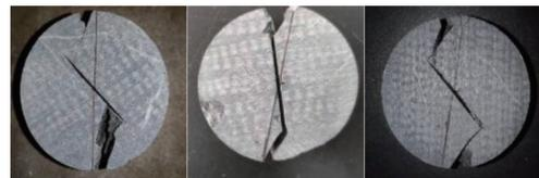
(c) 单裂隙试件30°加载
