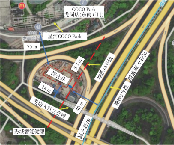
图1 综合井与邻近建(构)筑物平面位置示意图 Fig. 1 Planar position diagram of comprehensive well and adjacent structures
