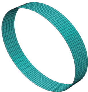
图 11 隧道盾构掘进阶段管片环有限元模型网格划分 Fig. 11 Mesh division of the finite element model of the segment ring in the tunnel shield excavation stage
