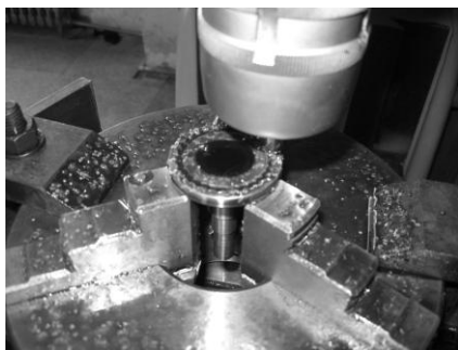
Fig. 8 The manufacture of cycloid tooth
