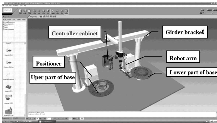
Fig. 2 The integrated model of welding robot system
