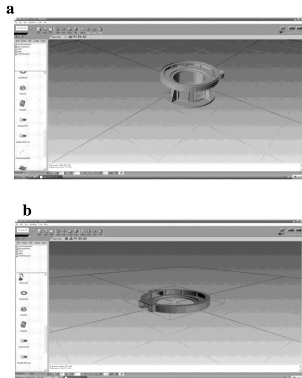
Fig. 1 Imported radar pedestal model of a) the upper part and b) the lower part
