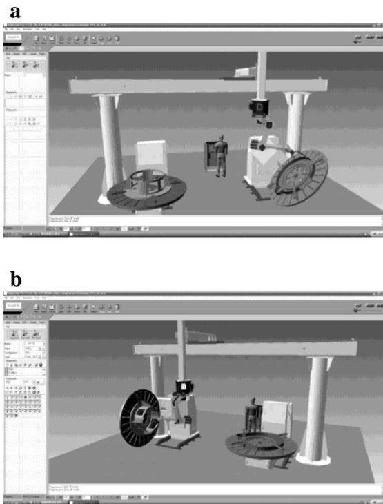
Fig. 3 Welding simulation of radar pedestal of a) the lower part and b) the upper part
