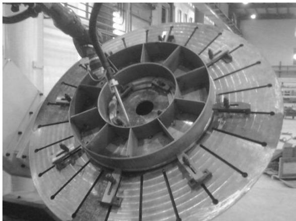
Fig. 5 Actual welding scene of welding robot
