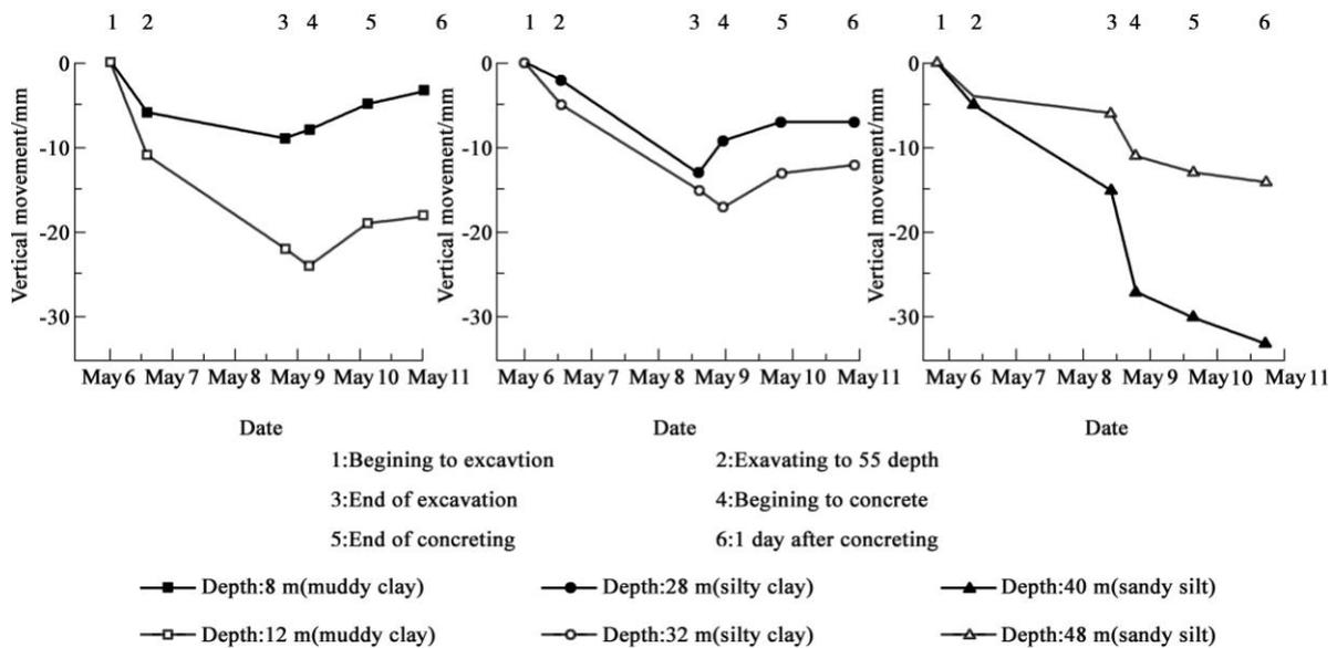
Fig. 17 Comparison of the soil displacement within different strata at different construction stages
