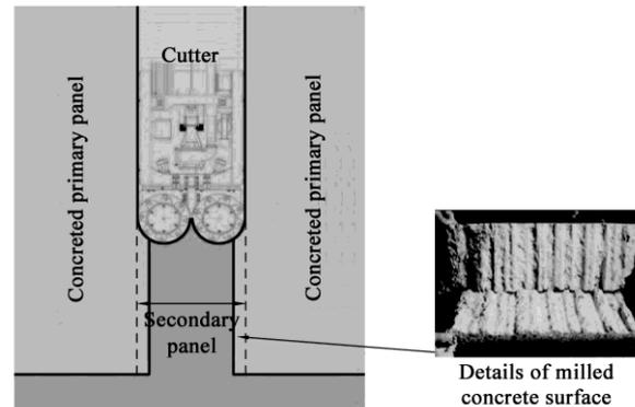
Fig. 3 The principle of overlapping method
