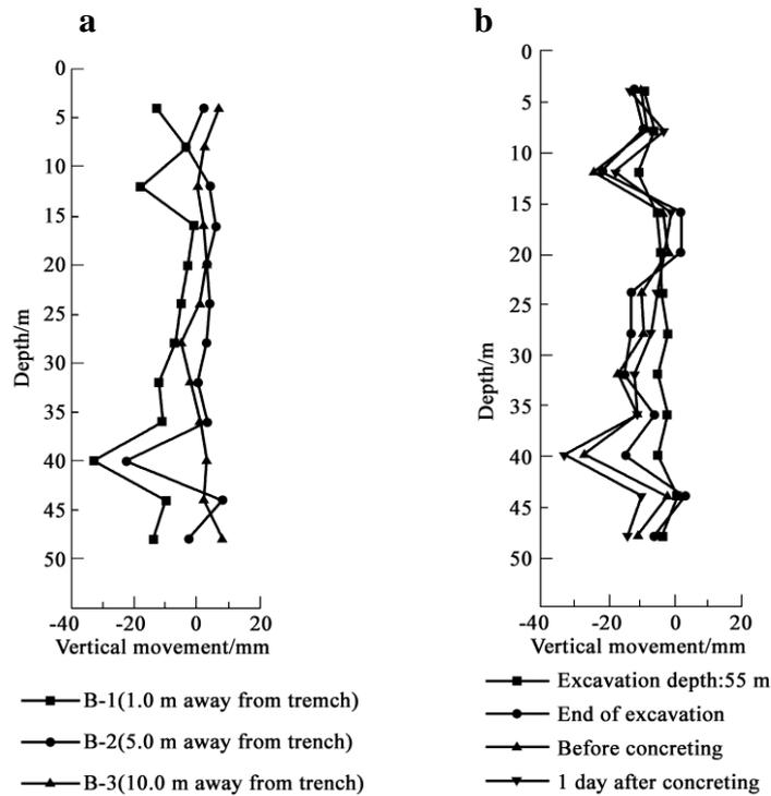
Fig. 16 Soil vertical displacement profiles: a) 3 boreholes 1 day after concreting; (b) different periods of B-1
