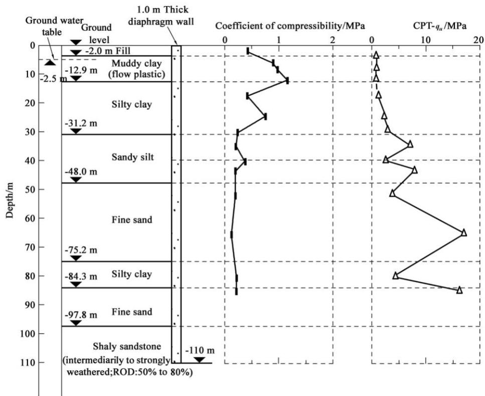
Fig. 2 Ground profile at the testing site
