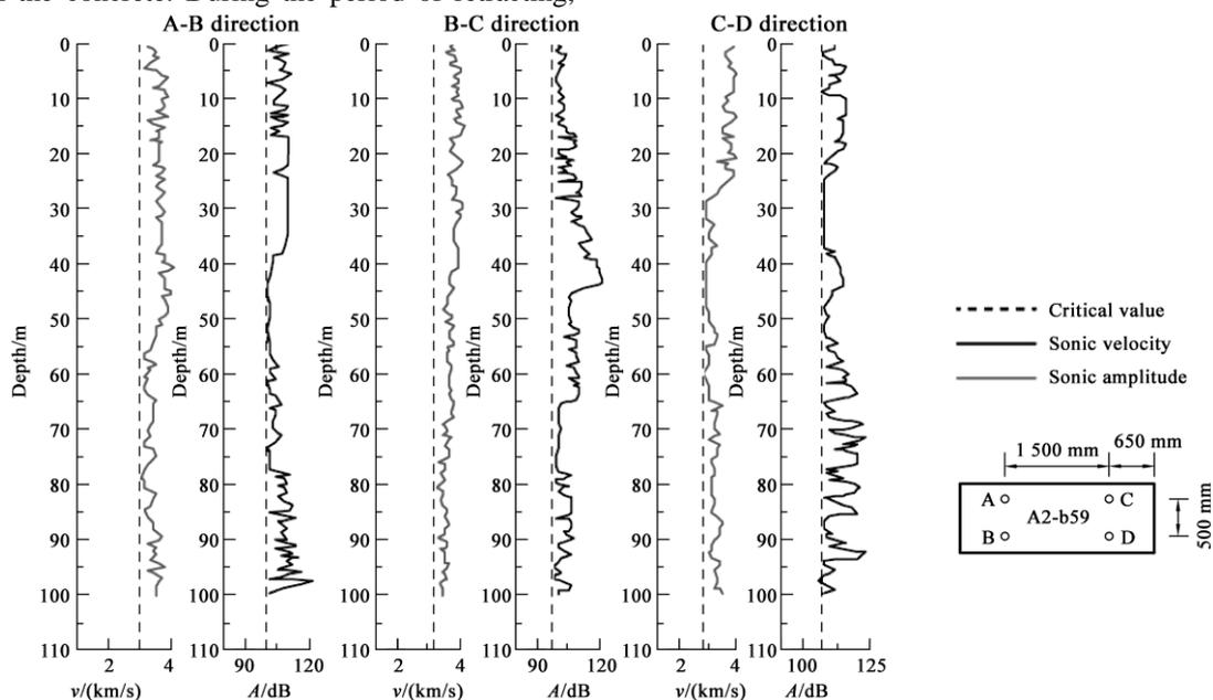
Fig. 11 Test result of the CSL (A2-b59), where  $v$  is the sonic velocity and  $A$  is the sonic amplitude
