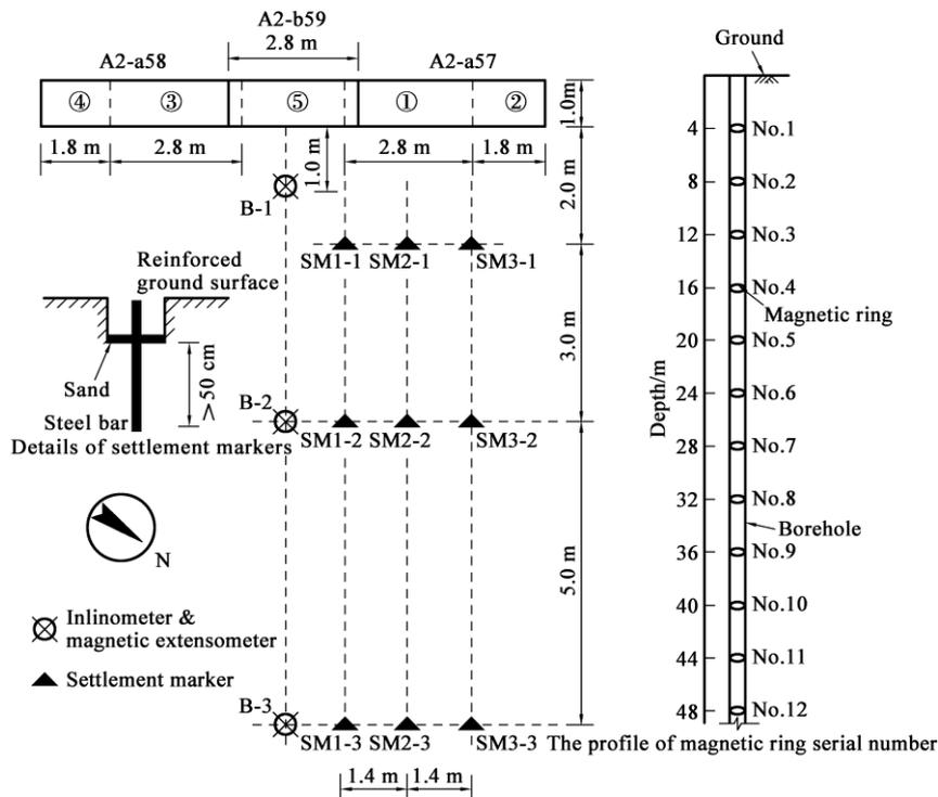
Fig. 12 Layout of the field testing program and monitoring instrumentation
