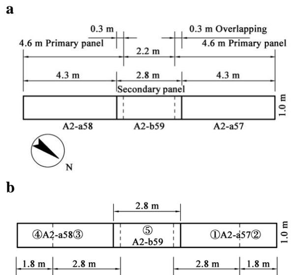
Fig. 4 The dimensions and excavation sequence of the three testing panels: a) Dimensions of three panels; b) excavation sequence of three testing panels
