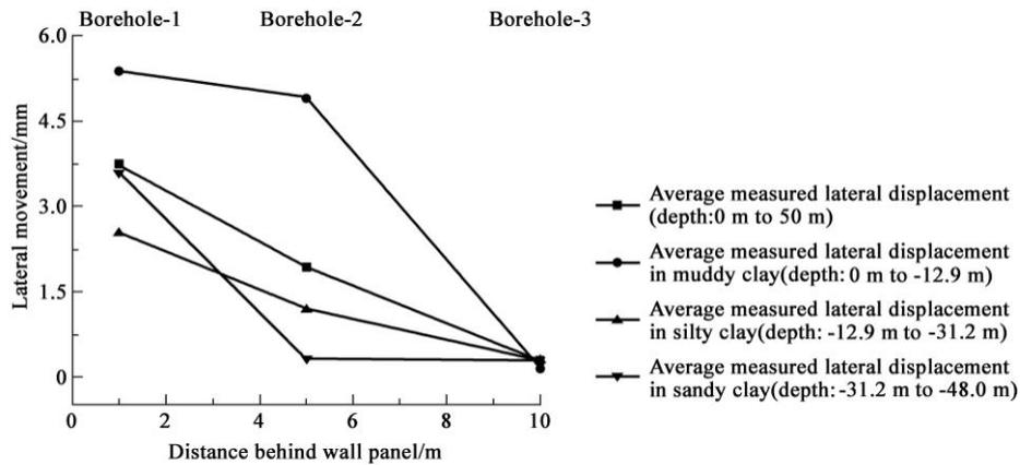
Fig. 15 Average lateral soil movement of different strata at various distances to the test wall panel
