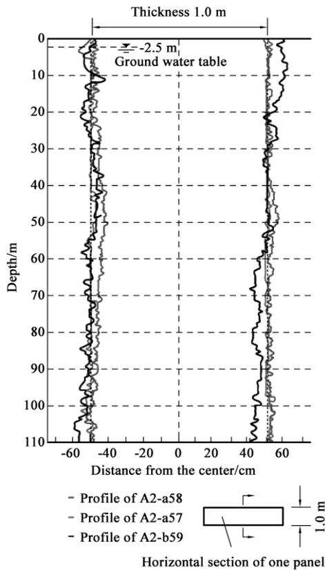
Fig. 9 Ultrasonic sounding profiles of trench faces
