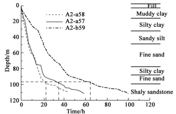
Fig. 10 Variation of excavation time of three panels with depth
