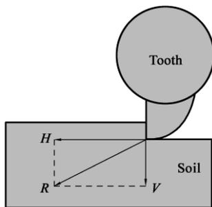
Fig. 7  $H/V$  ratio of the cutter teeth of a trench cutter [23]
