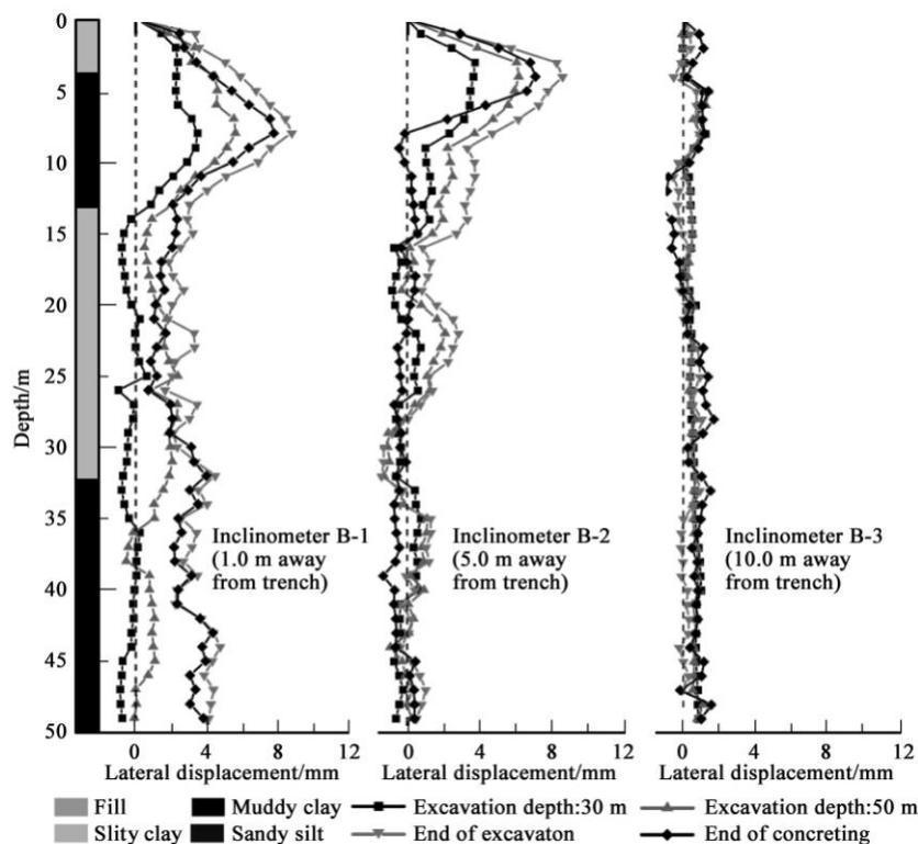
Fig. 14 Lateral ground deformation at different stages of diaphragm wall construction, where a positive value refers to a displacement toward the trench
