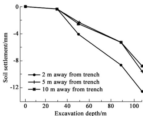
Fig. 13 Comparison of the soil surface settlement along trenching depth at different locations
