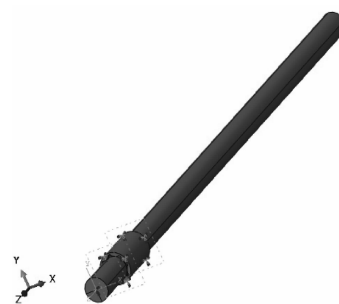
图2 水润滑橡胶轴承系统的载荷与约束 Fig.2 Load and boundary condition of bearing system
