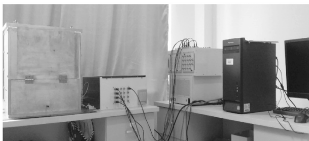
图 7 基于 dspace 的芯片固化炉实验系统 Fig.7 Experimental system of chip curing furnace based on DSPACE
