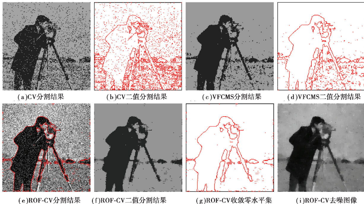
图6 噪声照相机图像的分割结果(噪声方差 \sigma=50 ) Fig.6 The segmentation results of noisy "Cameraman" image (noise variance \sigma=50 )
