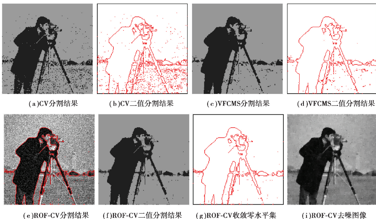
图5 噪声照相机图像的分割结果(噪声方差 \sigma=30 ) Fig.5 The segmentation results of noisy "Cameraman" image (noise variance \sigma=30 )
