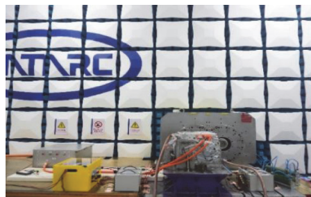
图 14 传导电压法测试布置图 Fig. 14 Test setup for conducted voltage method
