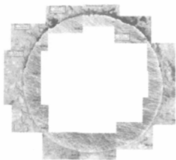
图 1 CorCha-A1 试样微观观测图 [10] Fig.1 Full corrosion distribution of specimen CorCha-A1
