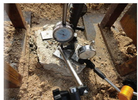
(c) 锚固体-周围岩体界面剪切滑移
