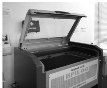
(b) 激光打印机进行构件切割
